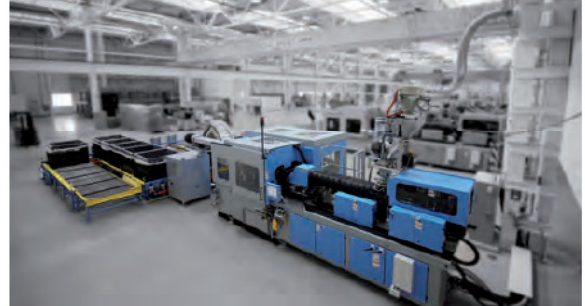
This 150t PET preform system serves as a Lightsout demonstration site for unattended moulding
