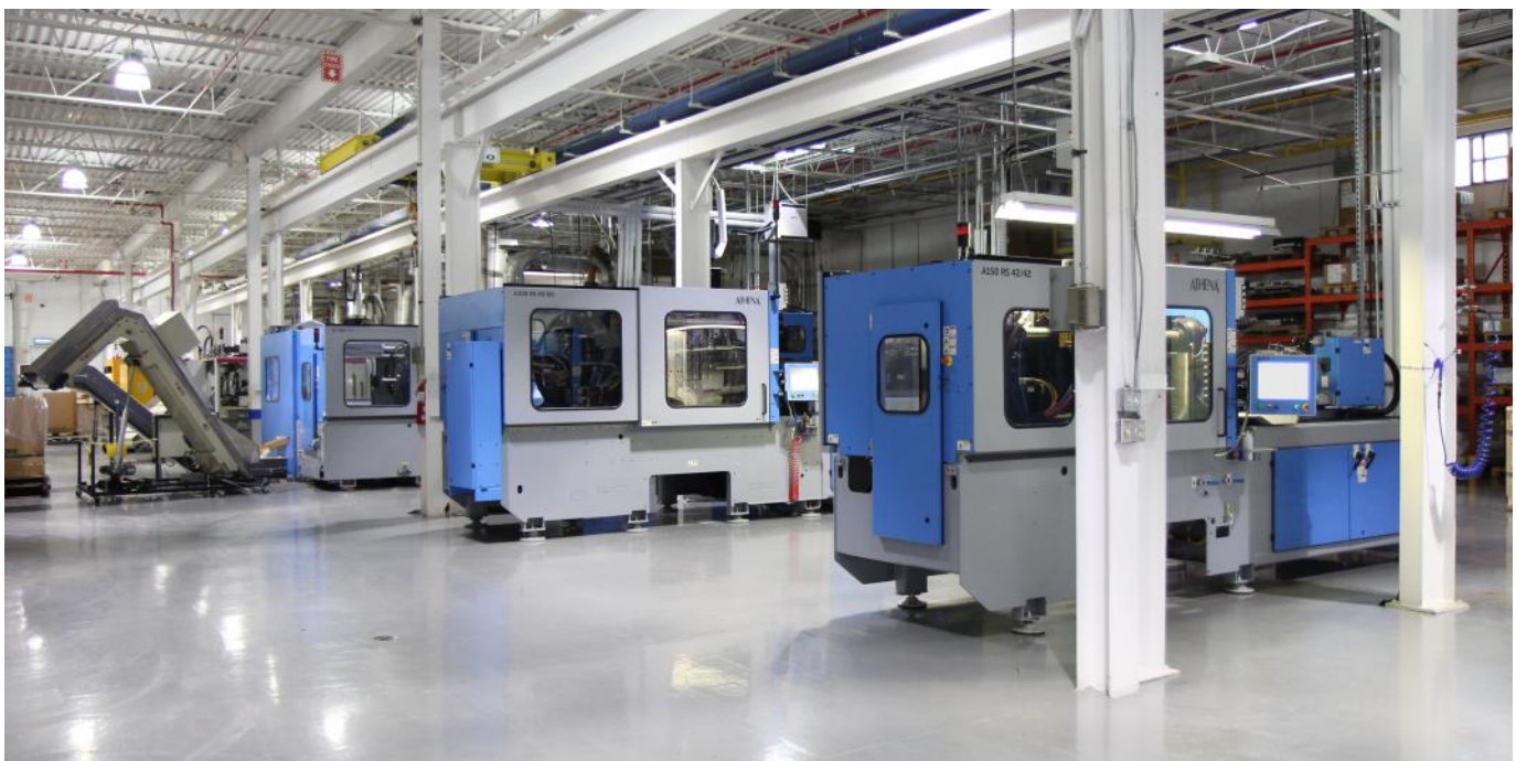
Cap-Thin's mold testing facility is equipped with a 150-ton and a 300-ton Athena machine
